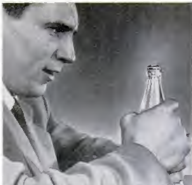
"Squeeze" the bottle to lift the coin on top. Moistened coin lifts when warmth of hands expands air in bottle and excess pressure is forced out past coin
